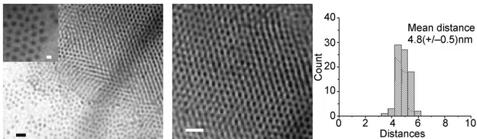
**Fig. 6** TEM of **Co2** as deposited on carbon graphite and distance histogram. Scale bar: main pictures 15 nm, insert: 3 nm.
