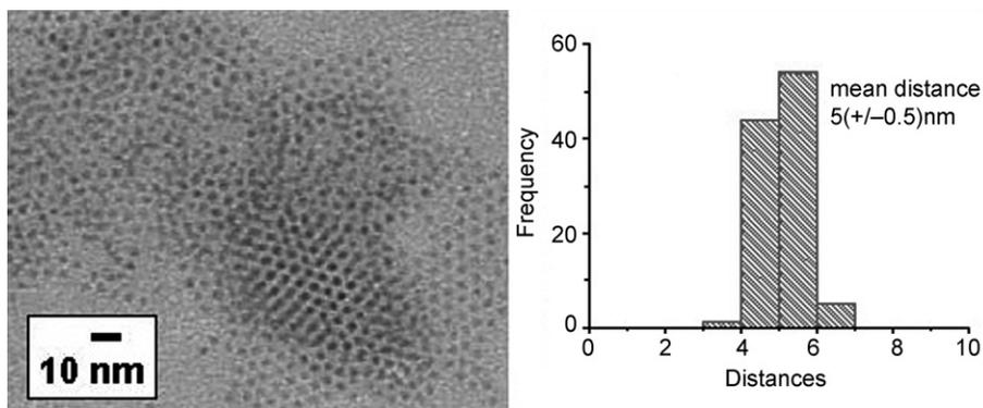
Fig. 2 TEM of cobalt nanoparticles stabilised by oleic acid, **Co2**, as deposited on amorphous carbon and distance histograms.
