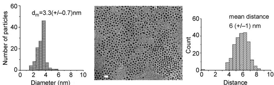
Fig. 3 TEM of hexadecylamine stabilised NiFe nanoparticles, **NiFe2**, as deposited on amorphous carbon, size and distance histograms. Scale bar: 10 nm.
