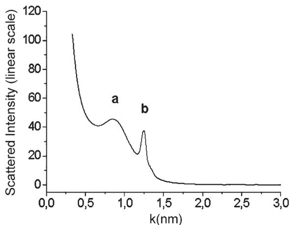
**Fig. 7** SAXS of **NiFe2** recorded at ESRF, beam line ID01,  $\lambda = 1.63 \text{ \AA}$  ( $a = 0.86 \text{ nm}^{-1}$ ;  $b = 1.25 \text{ nm}^{-1}$  corresponding respectively to distances of 7.3 nm and 5 nm).
