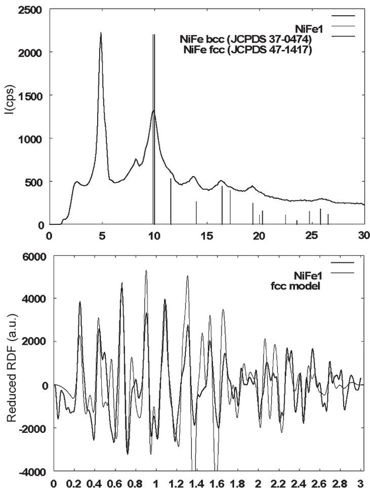
**Fig. 5** Top: Diffraction pattern for NiFe1, peak positions and intensities for two NiFe crystalline samples (JCPDS files converted to molybdenum wavelength); bottom: Radial distribution function for NiFe1 (full line) and computed from a spherical model (3 nm diameter) of FCC lattice (dotted line).
