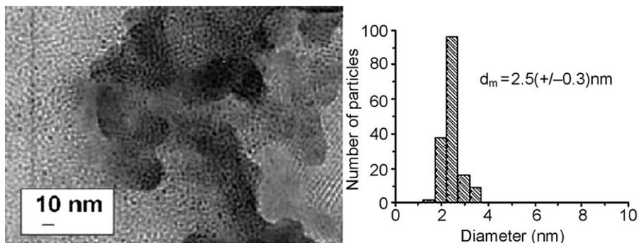
**Fig. 1** TEM of cobalt nanoparticles stabilised by oleic acid, **Co1**, as deposited on amorphous carbon and size histogram.
