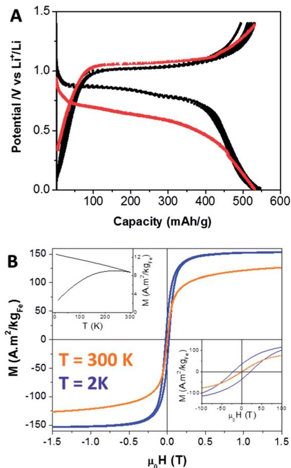
Fig. 2 Electrode potential vs. lithium during galvanostatic cycling for the *in situ* cell (red dots) and *ex situ* coin cell (black dots) (A); *ex situ* magnetic measurements after the 8<sup>th</sup> delithiation: hysteresis at 2 K (blue) and 300 K (orange), magnification of the hysteresis (right down panel) and ZFC/FC (left upper panel) (B).
