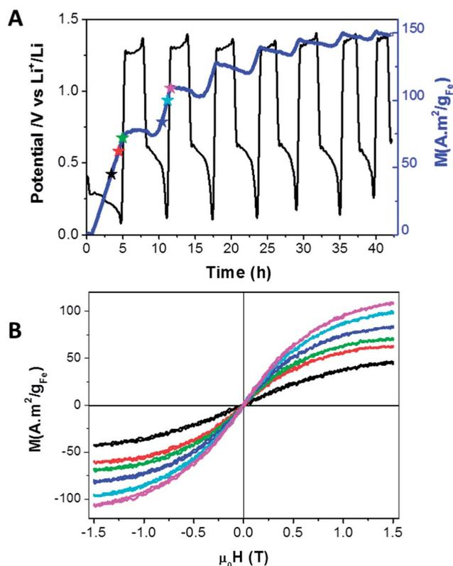
Fig. 3 Electrode potential vs. lithium during galvanostatic cycling of the *in situ* cell (plain line) and magnetic moment collected *in situ* at 300 K (blue dots) (A); *in situ* field dependent magnetic measurements; the different colors correspond to the stars on panel A (B).
