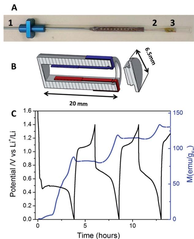
Fig. 1 Photograph of the inset for SQUID measurement (1), the electrical connections (2) and *in situ* cell (3) (A); schematic of the *in situ* cell (B); electrode potential vs. lithium during galvanostatic cycling (black) and corresponding magnetic moment at 300 K (blue) (C).
