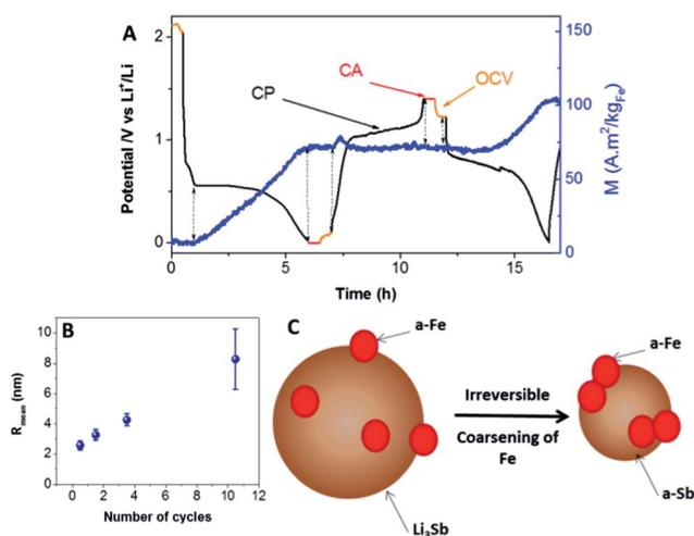
Fig. 4 Electrode potential vs. lithium during galvanostatic cycling for the *in situ* cell (black line), open circuit voltage (orange line), constant potential (red line) and magnetic moment at 300 K (blue dots) (A); magnetic particle size calculated from the *ex situ* ZFC/FC measurements as a function of the number of cycles for fully lithiated electrodes (B); schematic of the magnetic size coarsening (C).
