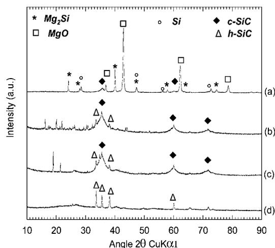
**Fig. 4** XRD patterns of SiC-SBA15 as-synthesised (a), after  $\text{H}_2\text{SO}_4$  treatment (b), after HF/EtOH treatment (c), and after thermal treatment (d).
