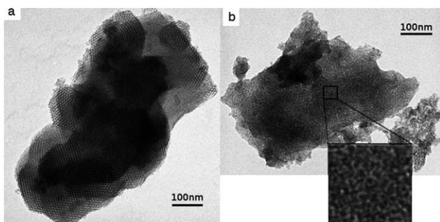
Fig. 5 TEM pictures of SBA15 silica material (a) and SiC-SBA15 (b).
