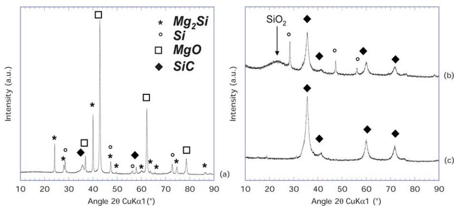
Fig. 1 XRD patterns of SiC-Stöber material as synthesized (a), after  $\text{H}_2\text{SO}_4$  treatment (b) and after EtOH/HF/ $\text{H}_2\text{O}$  treatment and thermolysis in air (c).
