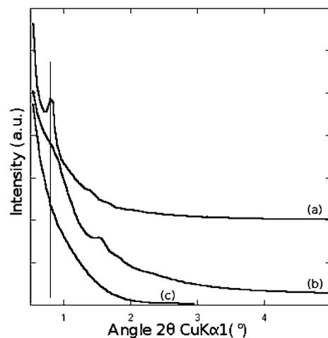
Fig. 6 XRD patterns at small angles for SBA15 silica material (a), C-SBA15 (b), SiC-SBA15 (c).
