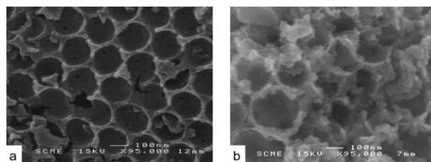
Fig. 2 SEM pictures of the mesoporous carbon (a) and the porous SiC (b).
