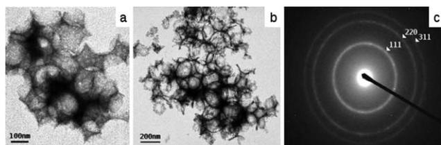
**Fig. 3** TEM pictures of mesoporous carbon (a), porous SiC (b) and electron diffraction on SiC (c).
