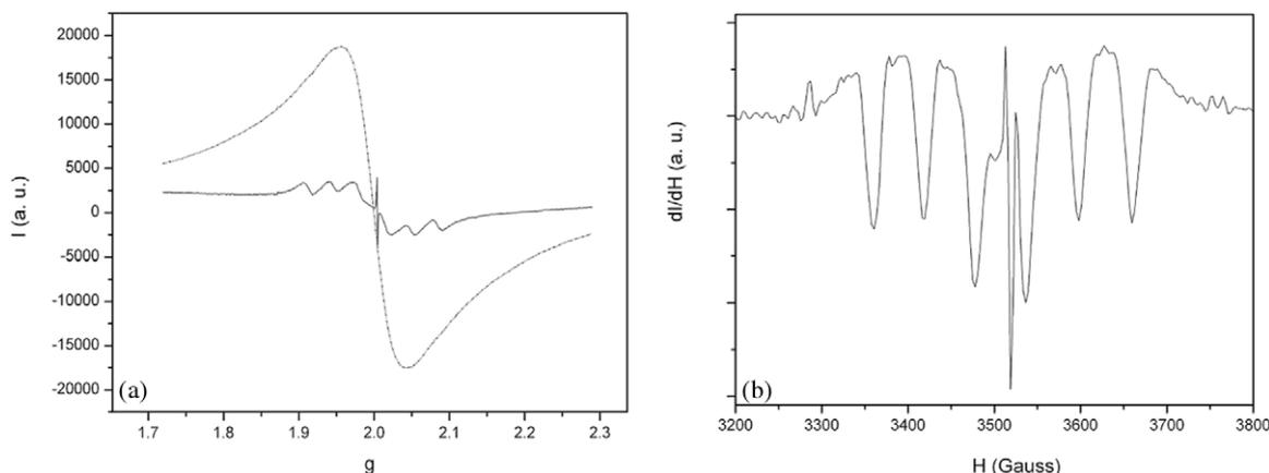
**Figure 4.** EPR spectra of  $\text{Cd}_{1-x}\text{Mn}_x\text{Te}/\text{C}$  samples at 300 K. Samples T1 (solid line) and T2 (dashed line) (a) and the first derivative of the EPR spectrum for sample T1.
