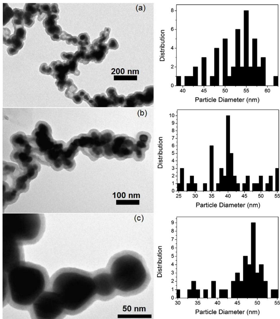
**Figure 2.** Bright field TEM images of (a) T1, (b) T2, and (c) T3, with the corresponding histograms of nanocrystal size distribution. The higher resolution of the T3 nanocrystals clearly demonstrates the core-shell morphology.
