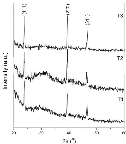
**Figure 1.** XRD patterns taken from the synthesized  $\text{Cd}_{1-x}\text{Mn}_x\text{Te}/\text{C}$  products.
