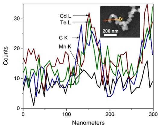
**Figure 3.** Elemental line scan of the nanocrystals in T3, as shown by an arrow in the SEM image (inset).
