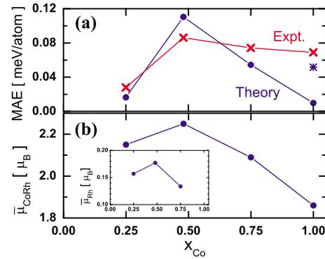
FIG. 2. (Color online) (a) Anisotropy energy and (b) average moment per CoRh unit  $\bar{\mu}_{\text{CoRh}}$  of 2 nm  $(\text{Co}_x\text{Rh}_{1-x})_N$  from experiment (crosses) and theory (dots,  $N=489$  atoms). The star refers to a dodecahedral cluster shape ( $x=1$ ). The inset shows the average moment  $\bar{\mu}_{\text{Rh}}$  induced at the Rh atoms.
