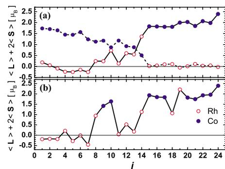
FIG. 1. (Color online) Local magnetic moments along the easy axis of 2 nm  $\text{Co}_{0.5}\text{Rh}_{0.5}$  clusters ( $N = 489$  atoms).  $j$  labels the nonequivalent atomic sites ordered by increasing distance to the central atom. (a) Fully segregated Co core with Rh shells (dashed) and Rh core with Co shells (solid). (b) Rh core with Co outer shells and intermixing at the interface.
