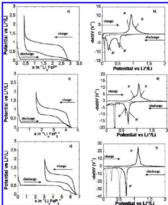
**Figure 2.** First cycles of FeP, FeP<sub>2</sub>, and FeP<sub>4</sub> electrodes versus lithium, plotted as the electrochemical potential vs the number  $x$  of lithium atoms inserted (a, c, and e for FeP, FeP<sub>2</sub>, and FeP<sub>4</sub>, respectively) and as the derivative  $-dx/dV$  vs potential (b, d, and f for FeP, FeP<sub>2</sub>, and FeP<sub>4</sub>, respectively). Dashed line: first discharge; solid line: first charge and second discharge.
