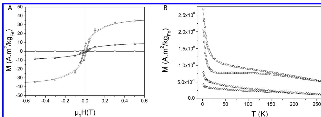
**Figure 7.** (A) Field dependence at 2 K of the magnetization of a  $\text{FeP}_4$  electrode (starting material: open circles) at various depths of lithiation after first discharge (open triangles), and second discharge (open squares). (B) Magnetic susceptibilities of  $\text{FeP}_4$  electrodes after first discharge (open triangles) and second discharge (open squares).
