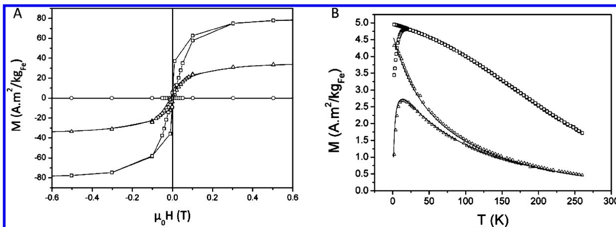
**Figure 6.** (A) Field dependence at 2 K of the magnetization of a  $\text{FeP}_2$  electrode (starting material: open circles) at various depths of lithiation after first discharge (open triangles), and second discharge (open squares). (B) Magnetic susceptibilities of  $\text{FeP}_2$  electrodes after first discharge (open circles) and calculated ZFC/FC (line).
