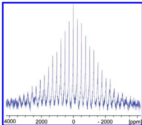
Figure 10.  $^7\text{Li}$  MAS NMR spectrum of  $\text{FeP}_2\text{-}4.3\text{Li}$  (116 MHz, 30 kHz spinning).
