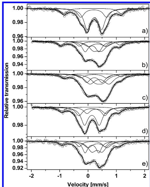
**Figure 5.** Mössbauer spectra of FeP<sub>4</sub> electrodes at various depths of lithiation; spectrum of the starting material recorded at 295 K (a), end of first discharge at 295 K (b) and 77 K (c), end of first recharge at 295 K (d), end of second discharge at 295 K (e).
