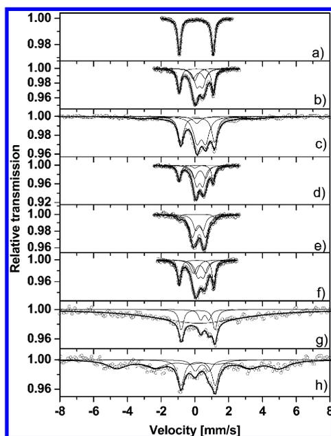
**Figure 4.** Mössbauer spectra of  $\text{FeP}_2$  electrodes at various depths of lithiation; spectrum of the starting material recorded at 295 K (a), end of first discharge at 295 K (b) and 77 K (c), half recharge at 295 K (d), complete recharge at 295 K (e), complete second discharge at 295 K (f), 75 K (g), and 20 K (h).
