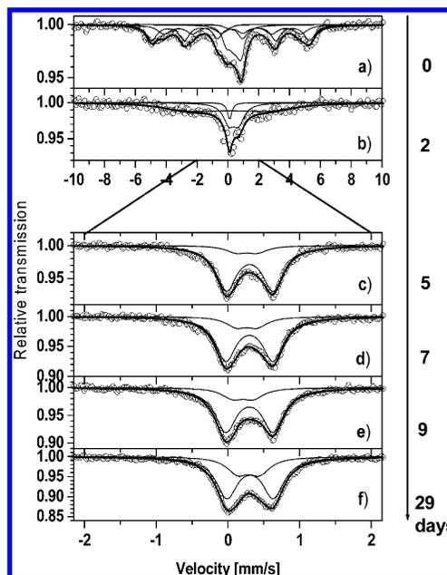
**Figure 13.** Evolution of a  $\text{FeP}$  electrode with time after two complete discharges. Mössbauer spectra recorded (a) immediately after the second discharge, and 2 (b), 5 (c), 7 (d), and 9 days (e) and 4 weeks (f) after the end of the electrochemical test. Spectrum (a) recorded at 77 K, and spectra (b–f) recorded at 295 K.
