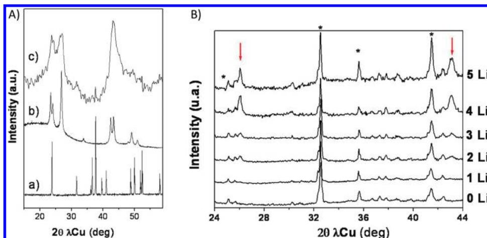
**Figure 3.** (A) X-ray powder diffractograms of (a)  $\text{FeP}_2$  starting material, (b)  $\text{Li}_3\text{P}$  obtained by mechano-synthesis, (c) a  $\text{FeP}_2$  electrode at the end of the first discharge. (B) X-ray diffractograms recorded in situ on  $\text{FeP}_4$  electrodes during the first discharge. The red arrows indicate main Bragg peaks of the ternary phase.
