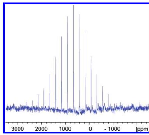
**Figure 9.**  $^{31}\text{P}$  MAS NMR spectrum for  $\text{FeP}_2-4.3\text{Li}$  (121 MHz, 30 kHz spinning).
