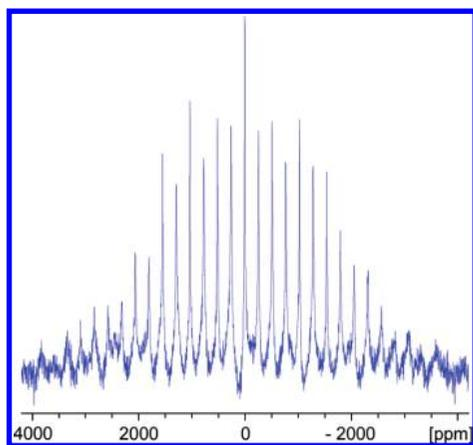
**Figure 8.**  $^7\text{Li}$  MAS NMR spectrum for  $\text{FeP}-2.3\text{Li}$  (116 MHz, 30 kHz spinning).
