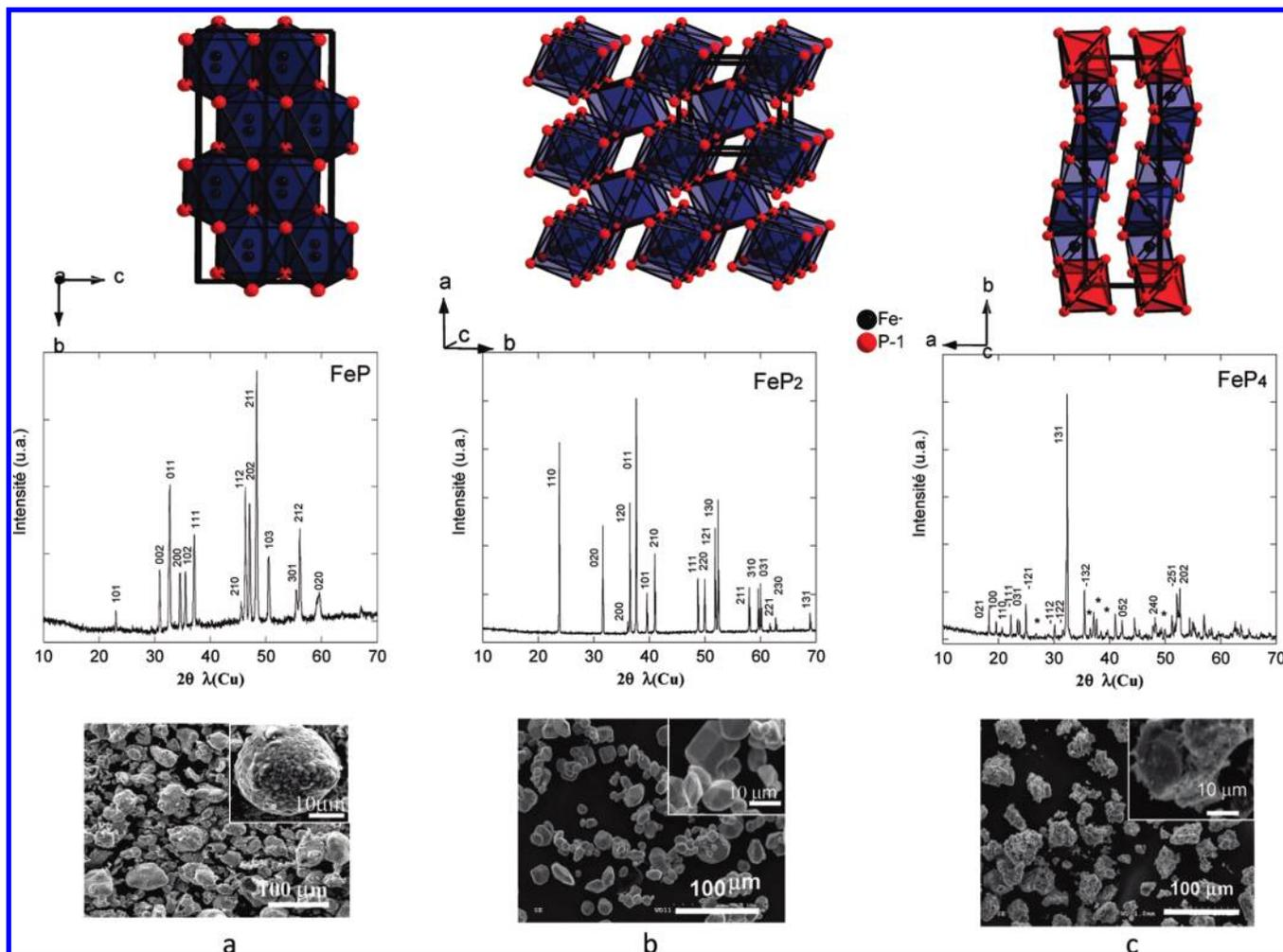
**Figure 1.** Powder X-ray diffraction pattern, SEM images and crystallographic cells of FeP (a), FeP<sub>2</sub> (b), and FeP<sub>4</sub> (c). Stars indicate the FeP and FeP<sub>2</sub> impurity traces in the FeP<sub>4</sub> pattern.
