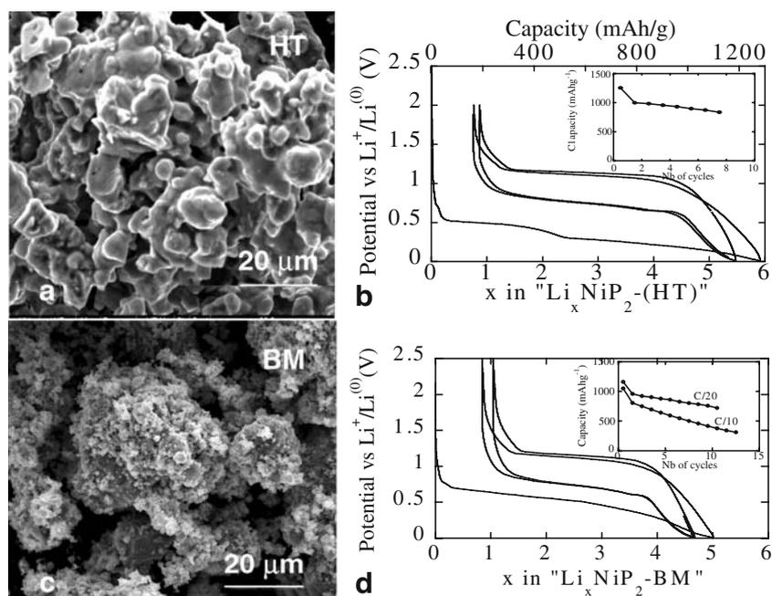
**Fig. 1** **a** SEM images of monoclinic  $\text{NiP}_2$  prepared by a high temperature ceramic route and **b** by a ball milling route. In **c** the voltage-composition traces for the HT- $\text{NiP}_2/\text{Li}$  and **d** for the BM-
